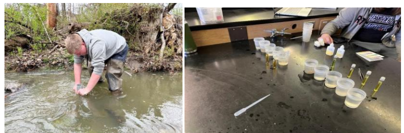
Figure 4. Sediment Core Sampling of macroinvertebrates (left) and water chemistry testing for nitrates and nitrites (right).
