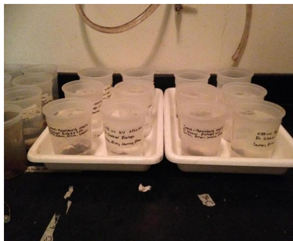
Figure 4. Lab setup of the pond snail bins as stored in Juniata College Ecology Department's laboratory fridge near native temperatures (~10°C). The bins in the left tray contained different concentrations of Kleen Up weed and grass killer and the bins in the right tray were different concentrations of Burn Out weed and grass killer.
